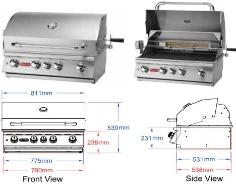
\*Red measurements shown are the recommended cut-out dimensions
